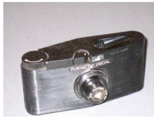
#34 Purma Special. 1937. 127 roll-film format. 12 square pictures per roll. Bakelite body with metal inner chassis. Spring-out precision lens. Streamlined design with viewfinder, shutter release, shutter tension and film wind-on all recessed into the body shell. Radical design of focal plane shutter. G.B.
