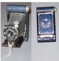
#21 . Girl Guide Kodak. 1931. 127 roll film format. Picture size: 6 x 4.5cm. All metal construction. Blue patterned finish. Girl Guide motif on front of lens panel and enamelled decal on track base. G.B.
