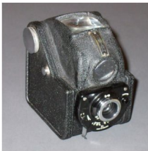
#11 Houghton Butcher Ensign 'Fulvue' camera post-war - 1945. 120 format roll-film. Picture size 6x6cm. Die cast all metal construction. Focussing lens. Radical body shape. Large meniscus reflex viewfinder. Up and under shutter release. G.B.
