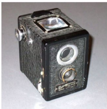
#10 Houghton Butcher Ensign 'Fulvue' Box camera. 1939. 120 format roll-film. Picture size: 6x6cm 12 per roll. All metal construction. Large meniscus reflex viewfinder and finding lens. G.B.
