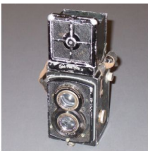
#12. Franke & Heideke Standard Rolleiflex camera. 1932. 120 format roll-film. Picture size 6x6cm. All metal precision construction. Reflex full size ground glass screen view-finding and focussing. Germany.
