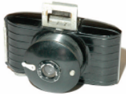
#28 Kodak Bullet Camera. 1936 127 format roll-film. Picture size: 1 5/8 x 2 inches. Bakelite construction with metal fittings. Large screw-out and lock lens mounting. Underside winding. Art deco styling. U.S.A.
