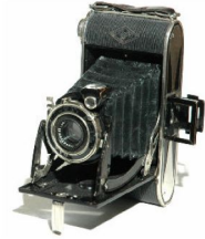
#17 Agfa Billy Record. 1933. 120 roll-film format. Picture size 6x9cm. Metal construction. Jgestar f8.8 precision anastigmat focussing lens. Rotating reflex viewfinder. Strut system brings lens out on opening. Action finder for eye-level use. Germany.
