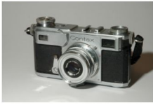
#24 Contax 11. 1936. 35mm film format. 36 exposures 36mm x 24mm. Interchangeable lenses. Wide base coupled rangefinder. Vertical drop metal focal plane shutter. Germany.
