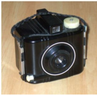
#26 Kodak Baby Brownie Special. 1939. All Bakelite construction. 127 roll-film format. Picture size: 1 5/8 x 2 inches. Moulded direct vision viewfinder. Art Deco styling. U.S.A.
